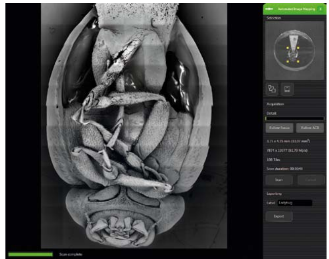
Figure 2: Example of large field of view automated image collection. The sample is a 3.15 x 4.15 mm ladybug that can be imaged completely at high resolution.
