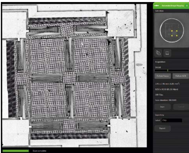
Figure 6 and 7: On the left: An overview of a 2.46 x 2.46 mm semiconductor scanned at high resolution, resulting in an 85 Megapixel image. On the right: A close up of the image map revealing small details on the surface of the chip.
