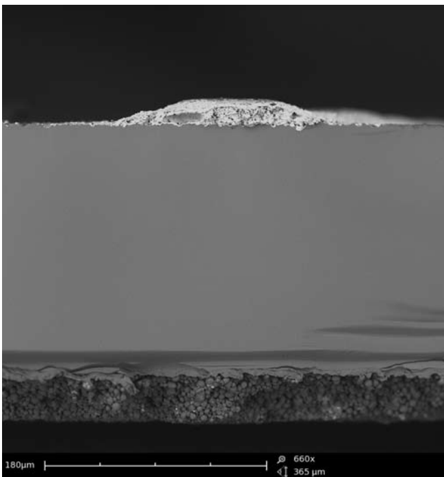
Figure 7: Cross-sectional image of solar cell showing top conductive track. These images are important in quality control for monitoring the exact dimensions and bonding of the track.
