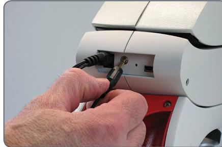
Both cables are now connected at the back of the Leica ICC 50.
