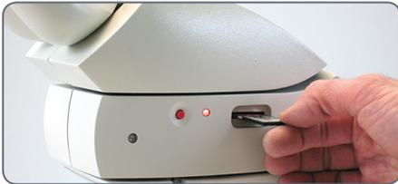
The camera's LED will turn green. The Leica ICC 50 is now ready to capture images onto the SD memory card.
