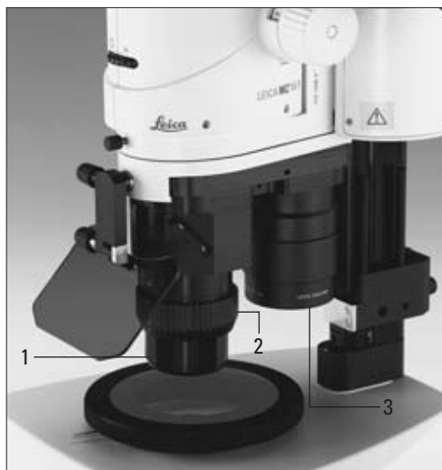
Fig. 16 HR planapo objective 5× rotated into the beam path
