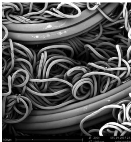
Figure 2. Elastic fibers embedded in nylon.
