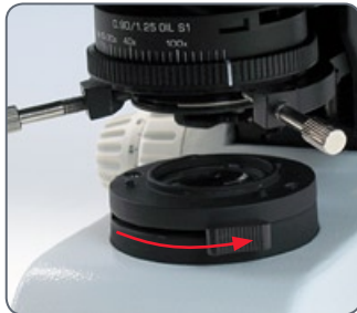
Close the Koehler field diaphragm
