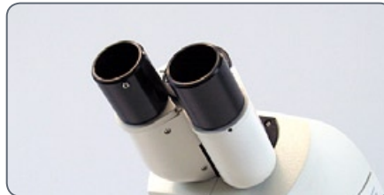
Type 2: Standard viewing tube with separate eyepieces
