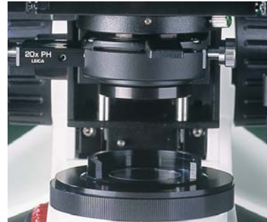
Superior critical or Koehler illumination
