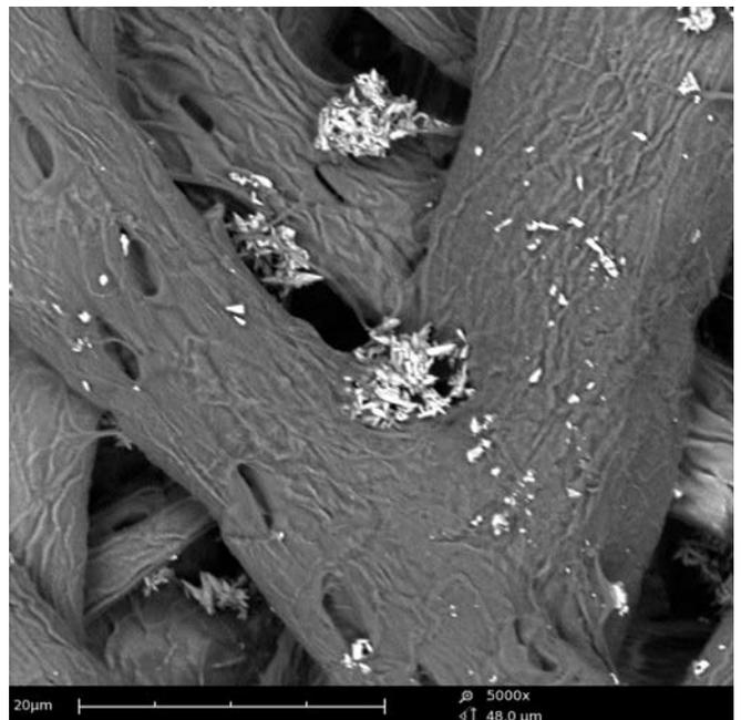
**Figure 4: Image of same paper using charge reduction sample holder. No charging is visible at 5000x magnification and image details are still clear.**
