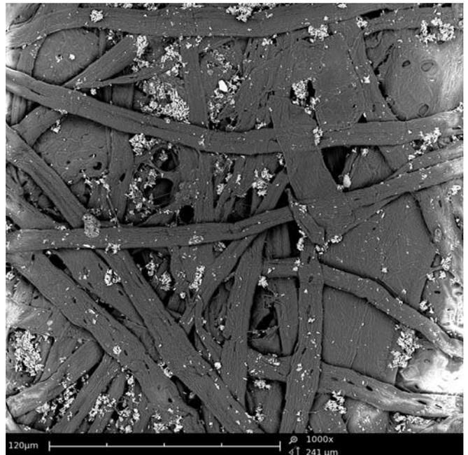
**Figure 3: Image of non-conductive paper. The image is taken using the standard sample holder at 1000x magnification. The bright white area's on both sides of the image is charging. At increased zoom, the charging becomes more localized and more distortion typically occurs until the image is completely obscured, yielding no data.**
