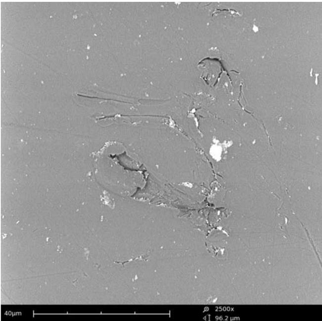
Figure 7: Defect in glass at 2500x magnification.
