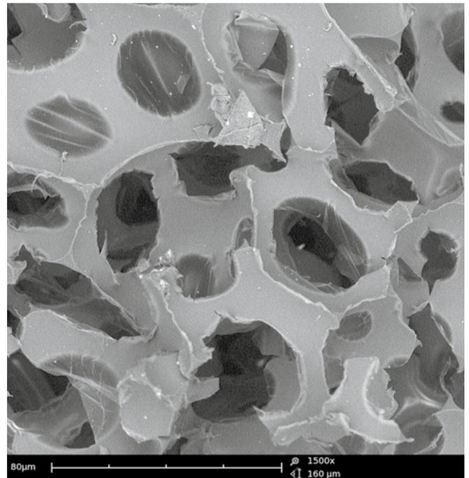
Figure 2: Polymer filter, 1500x magnification, imaged in its original state.
