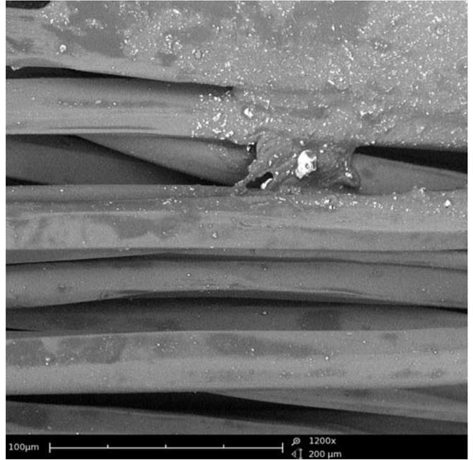
Figure 6: Coated textile fibers at 1200x magnification.
