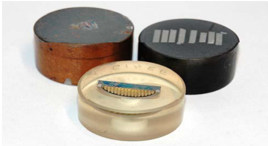
Metallurgical Charge Reduction Sample Holder
