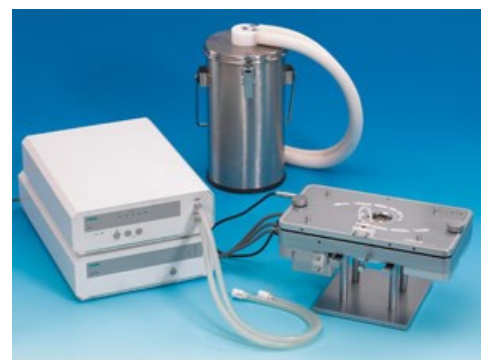
Low temperature Cryo-CSS450 system including dewar
