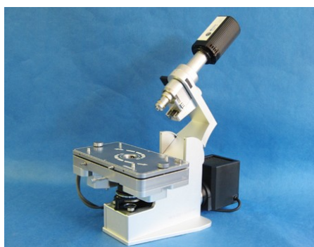
CSS450 stage mounted on the Linkam Imaging station. Sample image shows polymer flow using polarized light and phase contrast 10X objective.
