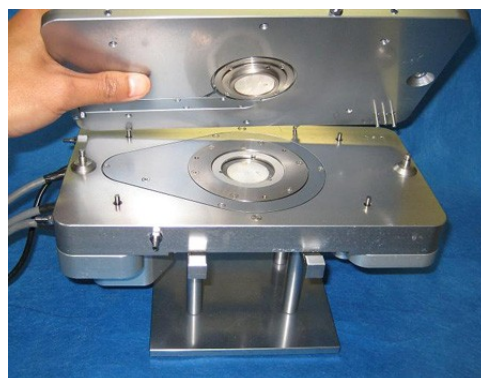
Lid of CSS450 being lifted off to reveal sample loading area
