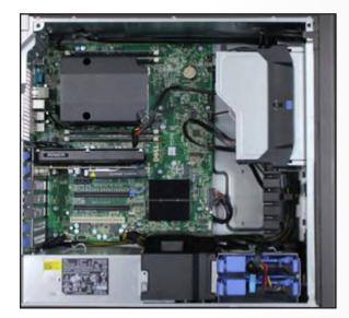
4. Locate an available 4 channel or higher PCIe slot (marked x4). Refer to the PC's documentation or side covers for motherboard's PCIe slots information.
