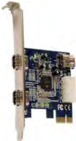
**Figure 3. FireWire interface Card**
