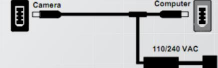
**WARNING:** Your camera will be damaged if the IEEE 1394 cable is not plugged into **BOTH** the computer **AND** the camera correctly. The cable connectors only fit one way and should slide easily into ports as shown below. Plugging the cable in improperly will void your warranty and require the camera to be returned to QImaging for repair.
