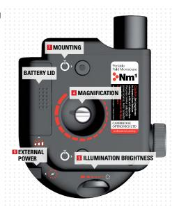
**ILLUMINATION BRIGHTNESS** ► The viewing brightness can be controlled by rotating the thumb wheel underneath for increased or decreased intensity in the direction indicated by the graphic.
