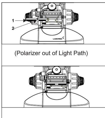
This high quality primary polarizer (1) is 360 degree rotatable with fiducial marking (2) for quick identification of Polarized / Cross Polarized positions.
