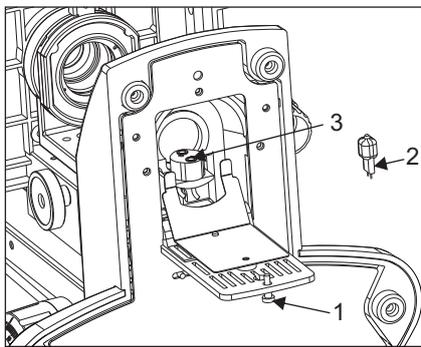
1. Before attaching the lamp bulb, remove the parts that may drop such as the filter and specimen from the Microscope frame, and place the Microscope on its back so that the bottom plate is exposed.
