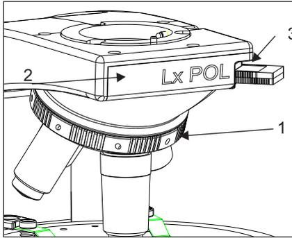
Swing in 10x objective in the light path. Adjust the condenser aperture diaphragm. Retrieve the two centering keys (Ref Fig 13 Part 5) and insert them in the centering holes (Ref Fig 10 Part 1) above the objective you want to center. Focus the POL sample.
