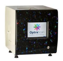
The OptraSCAN OS-FL Fluorescence scanner is an automated whole slide scanner with 15 sample slide capacity. A brightfield and fluorescence scanner, with five user changeable filters. Zoom from 1x to 750x without changing objectives. High speed stage allows extremely fast fluorescence scanning. Touch screen integrated computer control. No keyboard, no mouse, intuitive use, simple, ingenious. IMAGEPath Image Management system included for viewing, storage and archiving. Bar code enabled.
