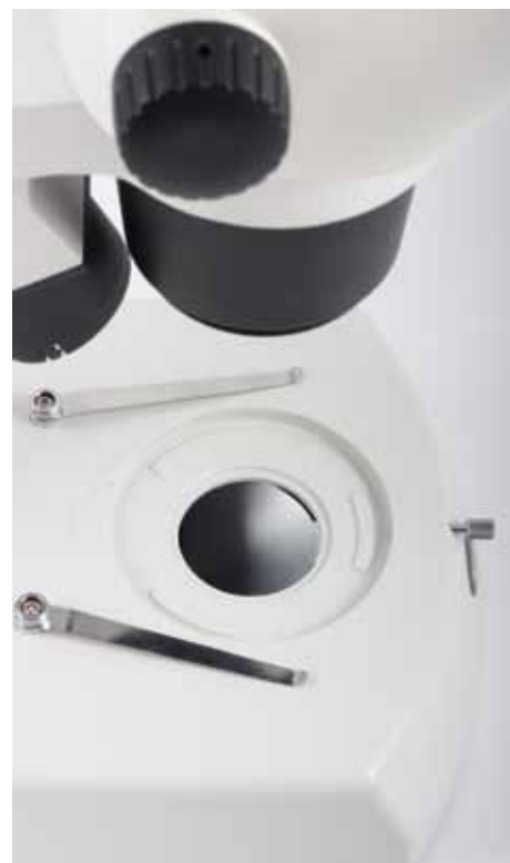
Built-in reflector for better illumination
